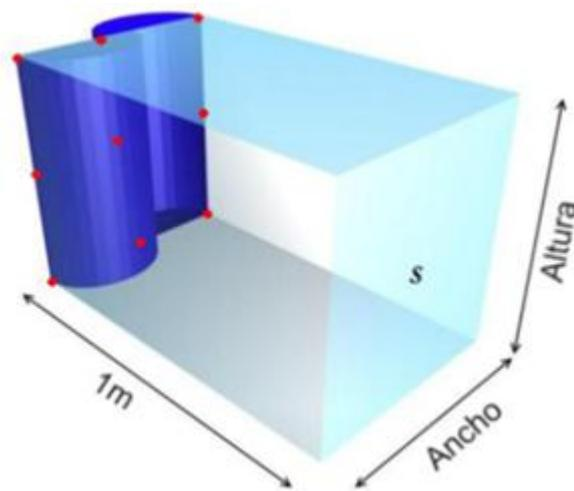
**Figure 9.** Measure points of wind velocity (in red) and attack surface (S) of wind turbines.
