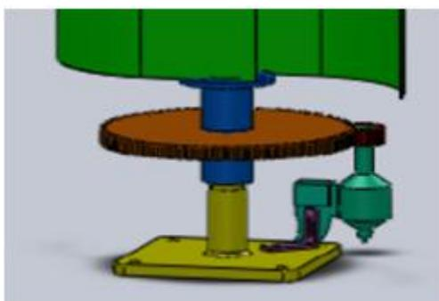
**Figure 3.** Set of base, axis, mass, transmission y generator.
