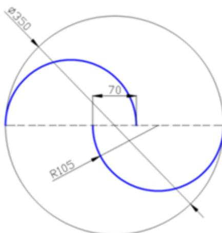
**Figure 4.** Savonius turbine cross section with measures.
