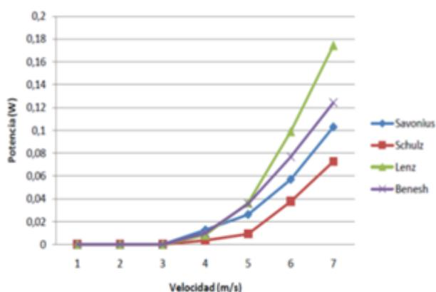
Figure 12. Power curves of the 4 wind turbines.
