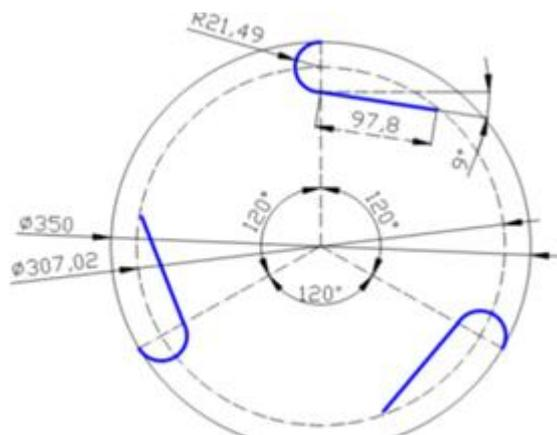
**Figure 7.** Lenz turbine cross section with measures
