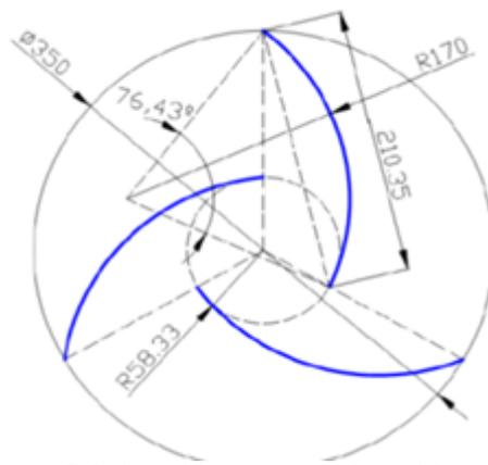
**Figure 5.** Schulz turbine cross section with measures
