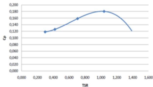
**Figure 10.** Power coefficient vs. specific velocity of the Savonius turbine.
