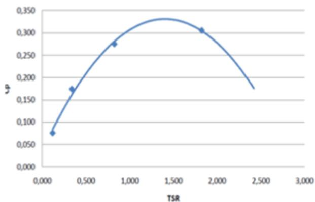
Figure 11. Power coefficient vs. specific velocity of the Lenz turbine.
