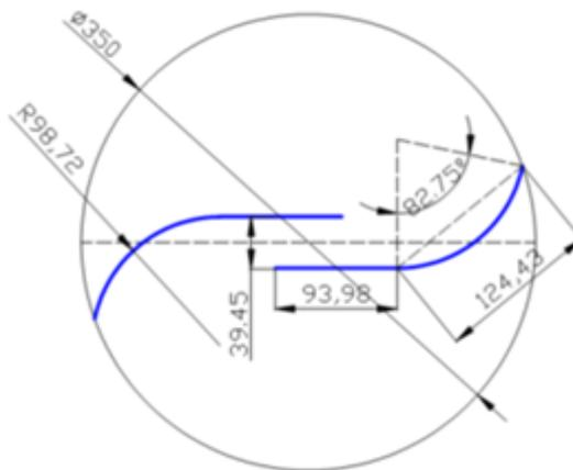
**Figure 6.** Benesh turbine cross section with measures.
